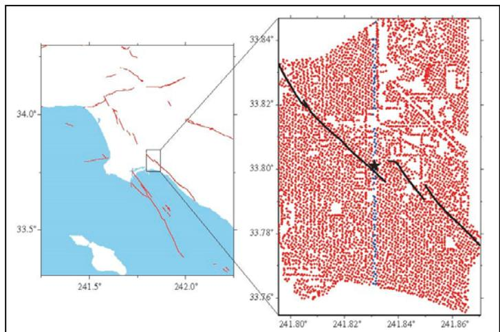
**Figure 1.** The layout of the Long Beach nodal array. There are over 5000 nodes in the array.
