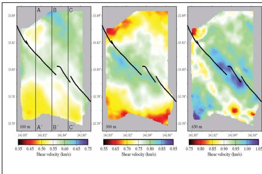
**Figure 2.** Shear wave results for layers at depths of 100m, 300m, and 650m are shown. The dark blue region highlights the Newport-Inglewood Fault structure, and the red zones show zones of low shear velocity near the coast, which are prone to liquefaction during earthquake shaking.
